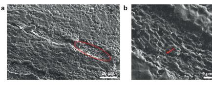
Figure 2. a) An SEM image of a 10  $\mu$ m thick coronal mouse-brain section on a NAPA chip after exposure to 10 laser pulses per position at a fluence of 100 mJ cm $^{-2}$ . Step size between the exposed areas is 50  $\mu$ m. The altered tissue as a result of laser desorption in a single pixel is highlighted by a red ellipse. b) Higher-magnification SEM image showing pores (see arrow) generated by tissue removal as a result of the hot nanoposts heated by the laser radiation.
